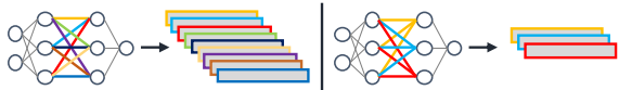
Figure 4.1.2: Trained NN weights are the input sequence to a transformer. Left. Each element in the sequence represents the weight that connects two neurons at two different layers. Right. Each element in the sequence represents the set of weights related to one neuron.
