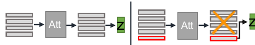
Figure 4.1.3: Multi-head attention-based encoder. Left. Regular sequence-to-sequence translation, each element of the output sequence is used. Right. An additional compression token is added to the sequence. From the output sequence, only the compression token is taken.
