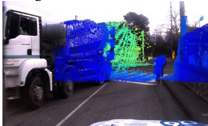
Fig. 7: LiDAR point cloud projected onto an RGB image in a dynamic scene.
