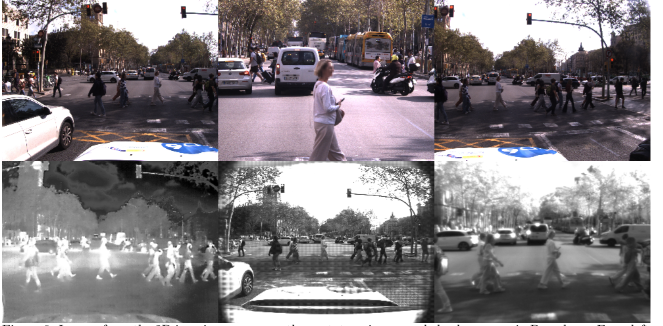
Figure 6: Images from the 2D imaging sensors on the prototype in a crowded urban scene in Barcelona. From left to right, top row: wide left, narrow, and wide right visible RGB cameras. Bottom row: thermal, polarimetric, and SWIR cameras.
