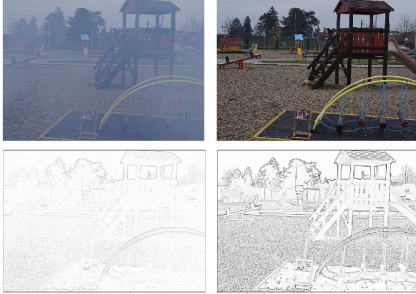
Figure 5. Gradient comparison between a fogged image (left) and its fog-free ground truth (right). Both colour images are presented on top with their associated edge images below.
