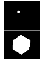
Figure 1. The same voxel in 3D space seen by a close camera and by a far one
