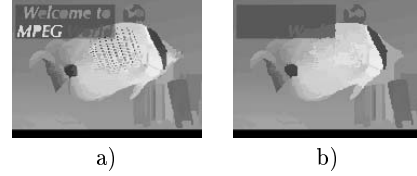
Figure 7: Size-oriented simplification. a) simple size simplification. b) size simplification with propagation strategy
