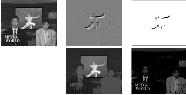
Fig. 3. Motion detection of maxima: Top row: original image, Middle row: temporal gradient, mask of the marker; Bottom row: anti-extensive reconstruction of the marker, difference between the reconstruction and the original images.
