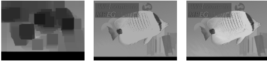
Fig. 2. Size filtering with opening by reconstruction: Left) erosion of the original bream image by a flat structuring element of size 10 \times 10 , Center) reconstruction of the erosion, and Right) second reconstruction.
