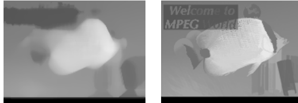
Fig. 5. Size filtering with leveling: Left) Median filter with a window of size 15x15 and Right) Self-dual reconstruction of the median filter.
