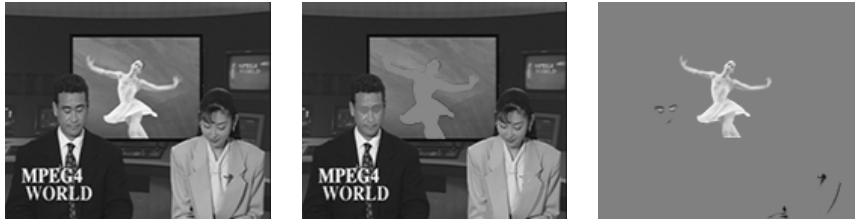
Fig. 6. Example of motion connected operator preserving fixed objects: original frame (left), motion connected operator (center), residue (right).
