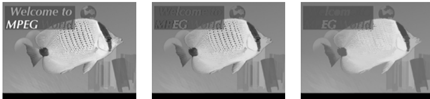
Fig. 3. Area filtering: original (left), area opening (center), area open-close (right).
