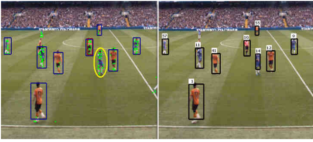
Figure 6 - The left image shows the detected person regions described by bounding boxes and tracked feature points. The resulting tracked persons with their bounding boxes and IDs are shown on the right.
