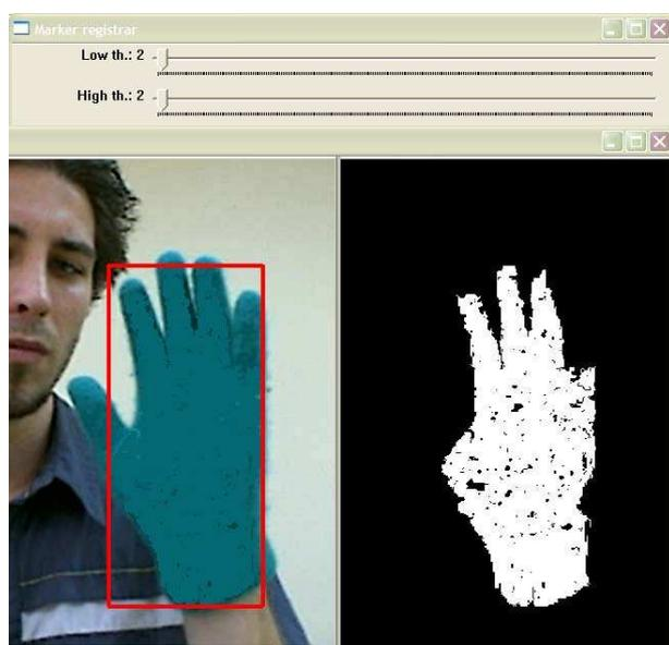
Figure 14: Effect of low settings for the floating range mode
