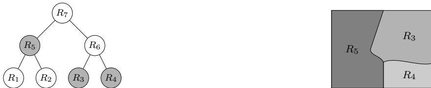
Figure 4: Lagrangian optimization over BPT. The bottom-up analysis follows the merging sequence from Fig. 1 activating the nodes with minimum lagrangian. The algorithm finds the best partition (regions 3, 4 and 5) and the best coding strategy.
