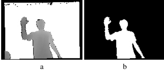
Figure 2. a) Depth map (depth maps shown in this paper are conveniently clipped and scaled for better visualization in grayscale images). b) Extracted silhouette.
