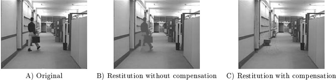
Figure 10: Example of restitution with (C) and without (B) motion compensation in the case of motion connected operators
