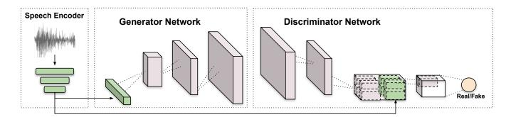
Fig. 1. The overall diagram of our speech-conditioned face generation GAN architecture. The network consists of a speech encoder, a generator and a discriminator network. An audio embedding (green) is used by both the generator and discriminator, but its error is just back-propagated at the generator. It is encoded and projected to a lower dimension (vector of size 128). Pink blocks represent convolutional/deconvolutional stages.
