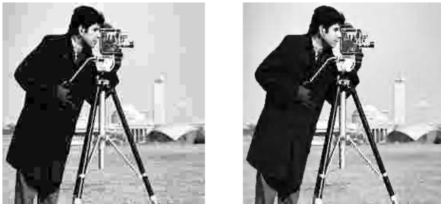
Fig. 8. Results: left, JPEG at 0.35 bpp; right, described technique at 0.33 bpp
