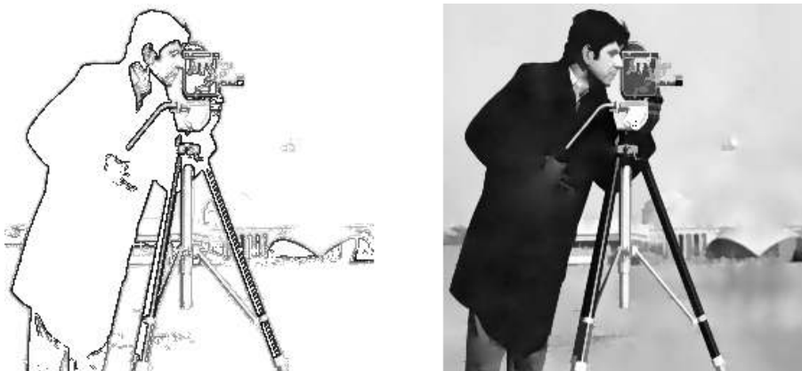
Fig. 5. Morphological interpolation from pixels with large Laplacian values: left, initial image (about 10% pixels); right, interpolation result
