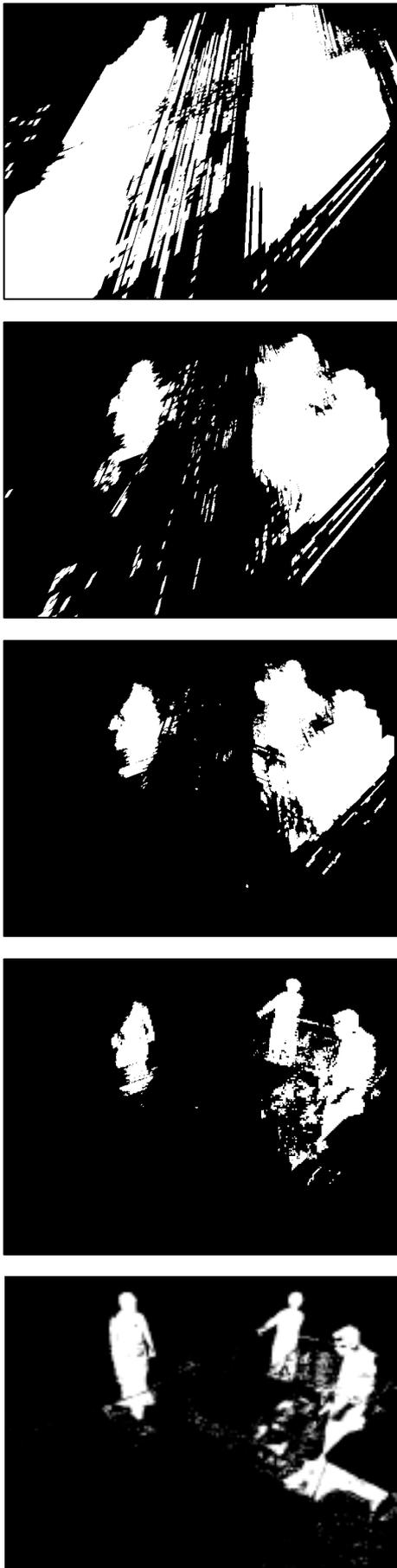
Figure 17: Results of progressive Shape-from-silhouette reconstruction with increasing number of cameras. From top to bottom: projection of the 3D reconstruction with 2, 3, 4 and 5 cameras. Bottom image: original (noisy) 2D foreground.
