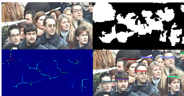
Figure 6. Partial occlusion. From left to right: original image, binarized skin-likelihood masks, skeleton transformation and detected faces.
