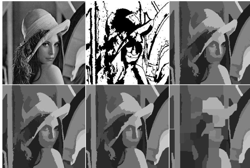
Fig. 9. Example of decision with the region growing version of the watershed. First row: original image, markers, decision with \alpha = 1.0 . Second row: decision with \alpha = 0.7 , decision with \alpha = 0.4 , decision with \alpha = 0.0 .
