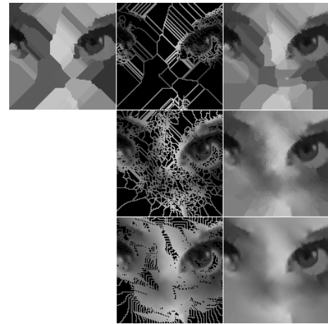
Fig. 19. Three iterations (2nd, 4th and 8th) of the geodesic propagation process, middle column: initial and secondary pixels, right column: propagation result.
