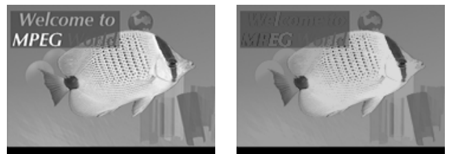
Fig. 2. Example of area opening. left: original image, right: area opening with size threshold equals to 500 pixels. The regional maxima of the filtered image have at least 500 pixels, but all minima and transition regions may be of smaller size.
