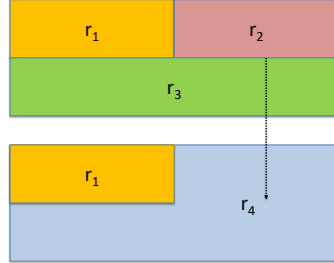
Fig. 7 The Single-View rate for each region is the rate saving promoted by the merging. Regions r_2 and r_3 are merged into r_4 , leading to represent the depth map without the contour between r_2 and r_3 and saving one 3D plane.
