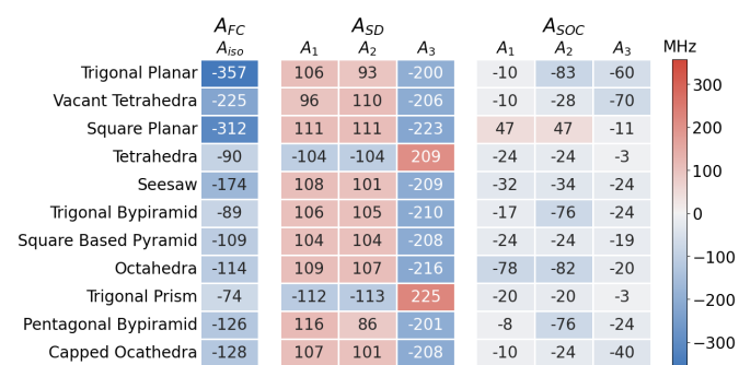
Figure 9. Heatmap of computed V^{IV} HFC components for [V(NH_3)_x]^{4+} (where x = 3-7 ) geometric model complexes. All calculations were performed using B3LYP/ANO-DK3 approach and using ZORA relativistic treatment.
