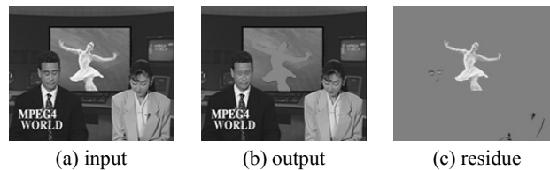
Fig. 5. Example of motion connected operator preserving still objects and its corresponding residue (input - output).
